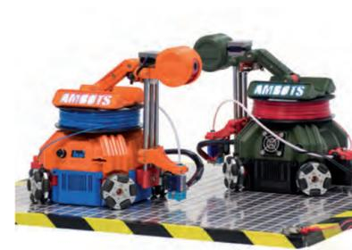
**Swarm 3D Printing and Assembly Robots**
